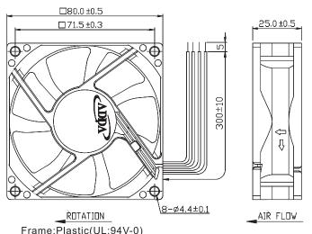
Frame:Plastic(UL:94V-0) Impeller:Plastic(UL:94V-0) Lead wire:UL1061AWG26
